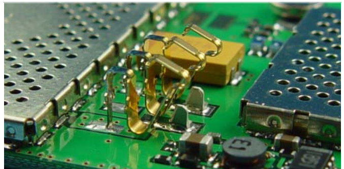
Desolder all pins and clean the pads.
