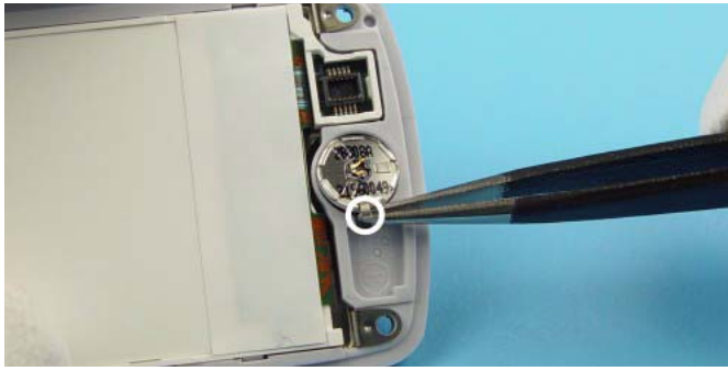
Remove Earpiece. Note the guiding pin when assembling.
