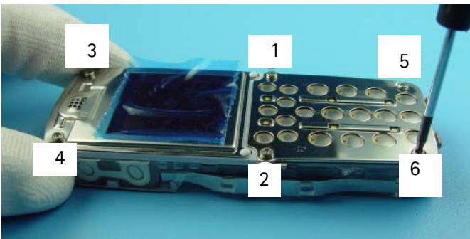
Tightening torques for screws (Note! Two tightening torques!): -screws 1-4, use 40 Ncm -screws 5-6, use 25 Ncm.
