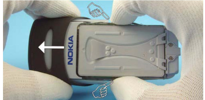
To remove the A-Shell press Locking Springs as shown and pull A-Shell from the unit.
