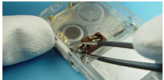
Use tweezers to remove Vibra Motor.
